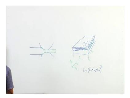
So, basically if you start there may be thicker material like this then there will be two rolls here like this and the material will go through that so that I will draw it like this ok. So, you have reduced the thickness of the material, but in this process what happens is you get a grain size that I will try to show you in three dimensions ok.
