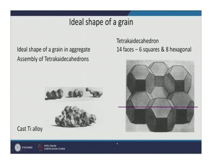
Ideal shape of a grain is called Tetrakaidecahedron ok, which has 14 phases which contains 6 squares and 8 hexagonal So, you can see one hexagonal here one square here another hexagonal here another square here and so on and some faces will be in the back. So, this is a kind of an ideal shape which you want to have for grains and which can give
