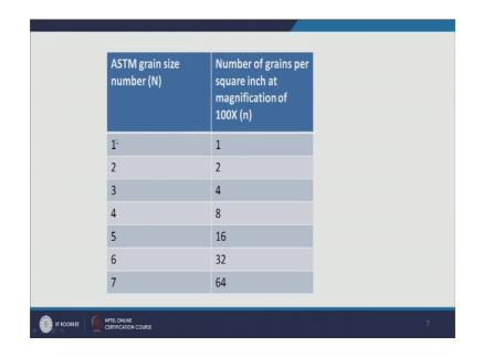
Then the number of grains per square inch at magnification of 100 x, which is a small n will be one if it is two then it is 2 of course, but if it is 3 then it will be four if grain size number ASTM grain size number is 4; that means, the number of grains in a square inch area will be 8.
