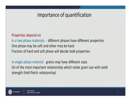
Let us say if you take two phase material, a different phases have different properties maybe one phase will be a softer phase. It can you can easily deform it another phase which is next to it may be a harder phase it is difficult to deform it and these two phases are in are together they are they are they there is an aggregate of these phases ok.
