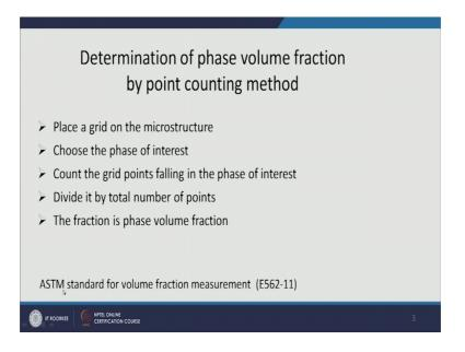
I will choose the phase in which I am interested for which I want to find out that how much is the fraction of that particular phase. Then I will count the grid points falling in
