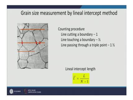
The idea is this, that if you get a microstructure as shown here in the slide you can see that there are grain boundaries and so on ok. Again a very simple method that you start putting some lines on the microstructure ok. For example, this middle line if you take; now we will count the number of intercepts this line is making with the grain boundaries ok.
