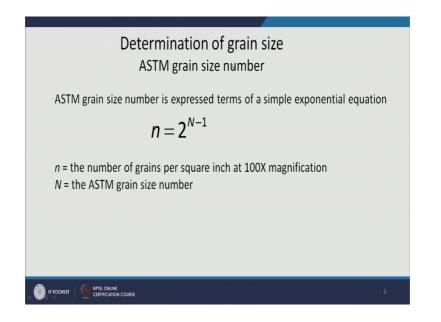
And that is actually a simple exponential equation given by an equation like this; a small n is equal to 2 to the power N minus 1, where a small n is the number of grains per square inch at 100 x magnification. So, in the microscope you set the microscope such that you are getting a 100 x magnification and in that 100 x magnification then you take a, a circle of a some, some area ok.
