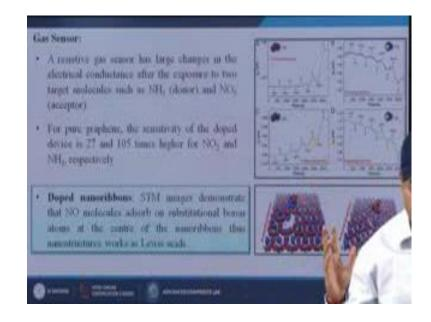
Here just we are going to show you that we are using 2 types of gases, one is the ammonia or maybe the ammonia environment, another one is the nitrogen dioxide or maybe the nitrogen dioxide environment. So, in this particular case, both are almost the toxic gases. So, in this particular case, what we are trying to do? We are trying to make our sensor so that easily it can detect this kind of gases. So, what we are trying to do over here.
