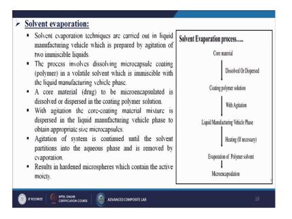
Next one is called the solvent evaporation methods. It is also a one kind of microencapsulation techniques. What this a techniques telling us? It is the techniques which are carried out in liquid manufacturing vehicle which is prepared by agitations of two immiscible liquids. So, simple two liquids which we are not mixing properly we can take for this particular purpose.
