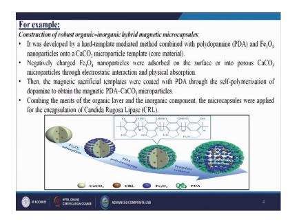
So, it is a one example just I am going to give so that we can better understand how we are doing the microencapsulation. So, it is example of a construction of robust organic inorganic hybrid magnetic micro capsules. So here, generally we are taking the polymer which is a nothing but the polydopamine and Fe 3 O 4 nanoparticle onto calcium carbonate microparticle templates which is known as the core material. Now, negatively
