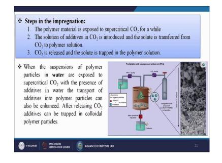
So, steps in the impregnations; how we are going to do this kind of techniques? The polymer material is exposed to supercritical carbon dioxide for a while. The solution of additives in carbon dioxide is introduced and the solute is transferred from carbon dioxide to polymer solutions. Carbon dioxide is released and the solute is trapped in the polymer solutions. So, this is the techniques.
