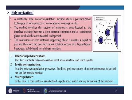
Next is called the simple polymerizations methods. It is also a randomly and most easily used method by which we can do the coating of our nanofillers or maybe any kind of core materials. So, what this process tells actually? A relatively new microencapsulation method utilizes polymerizations techniques to form protectives microcapsules coating in situ.
