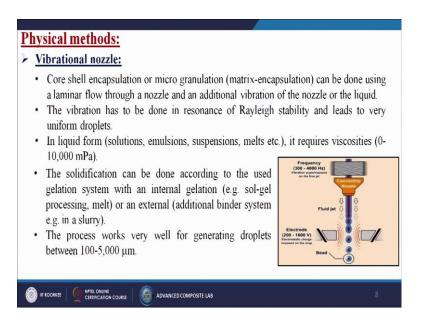
So, now fist we are going to do or maybe we are going to discuss only about the physical methods and fist one is the vibrational nozzle. So, in this particular you can see that we are having some kind of concentrating nozzle in which the high fluid is coming, then we are having some electrode and due to that frequency or may be that voltage potential difference that fluid is divided into small small parts or may be the small small bobbles or may be particular.
