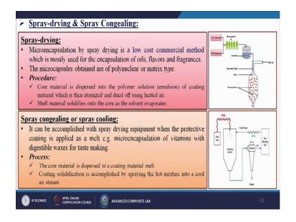
Now, next one we are going to discuss about the spray drying and spray congealing. So, in the spray dying process microencapsulation by spray drying is a low cost commercial method which is mostly used for the encapsulation of oils, flavors and fragrances. Generally we can use this one for our cosmetics products or maybe this one for our some food products or may be some other meals.
