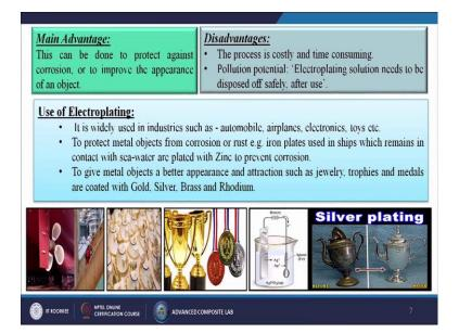
So, main advantage this can be done to protect against corrections or to improve the appearance of an object what are the disadvantages the processes costly and time consuming. Pollution potential electroplating solutions need to the disposed of safely
