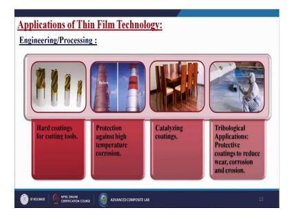
So, what at the applications of that thin film technology, engineering processing? Generally we are using for this materials for the hard coatings for cutting tools. So, generally we can do the coatings only the cutting regions so that the tool will be in expensive. Not only that sometimes we can change the carting geometric of this particular tool by using different types of inserts, that inserts can be made by different types of coating techniques.
