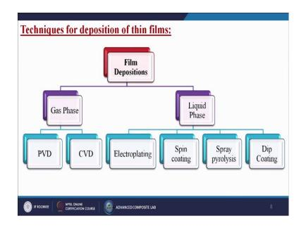
So, what are the techniques of deposition on thin films? Generally it can be divided into two parts: one is called the gas phase and other one is called the liquid phase. Gas phase generally you have discussing about the PVD process; physical vapour deposition process, and the CVD is call the chemical vapour deposition process. If you remember we have discussed the PVD process and our CVD process in details on lecture number 12 and lecture number 13.
