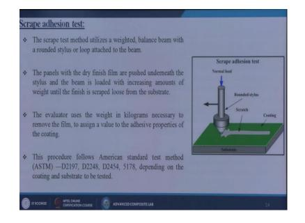
First one is called the scrap adhesion test; in the scrap test method utilizes a weighted balance beam with a round stylus or loop attached to the beams. So, it is known as the stylus in which we are putting a constant normal load either that load may be constant or may be it can be progressive and here so, we are starting the experiment from here then we are giving motions into these directions so, what will happen? This stylus or maybe that tip will rub onto the coating materials.
