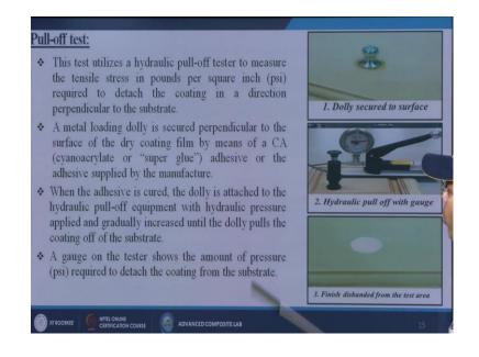
What is this? This test utilizes a hydraulic pool-off tester to measure the tensile stress in pounds per square inch psi required to detach the coating in a direction perpendicular to the substrate. A metal loading dolly is secured perpendicular to the surface of the dry coating film by means of CA, CA is nothing but the cyanoacrylate or maybe the super glue adhesives or the adhesive supplied by the manufacture.
