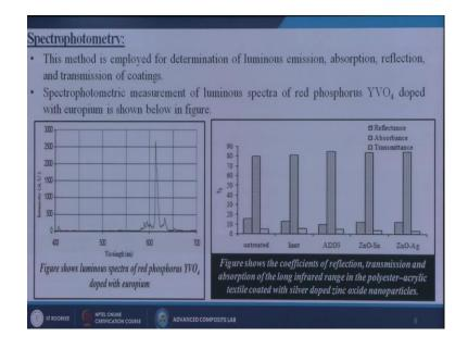
Next we are talking about the spectrophotometry. So, spectrophotometry this is also one kind of method which is employed for determination of luminous emissions absorptions reflections and transmissions of the coating. So, spectrophotometry; by using these techniques we can measure that luminous emissions, absorptions, reflections and transmissions of that particular coating materials. Spectrophotometric measurement of
