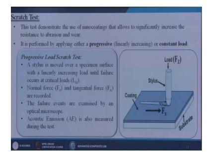
These tests demonstrate the use of nanocoatings that allows to significantly increase the resistance to abrasions and wear, it is performed by applying either a progressive, linearly increasing or a constant load.
