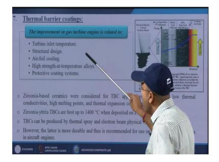
So, the improvement in gas turbine engine is related to turbine inlet temperature, structural design, airfoil cooling, high strength at a temperature alloys, protective coating systems. So, from this particular system you can understand that we are using these materials for a higher temperature; at a higher temperature then what we are trying to do we are using some kind of zirconia based ceramics were considered for the t v c
