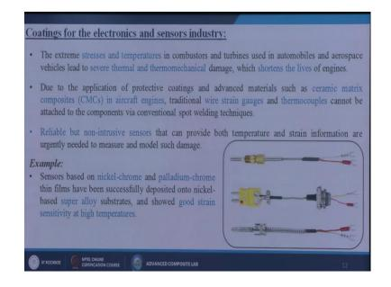
So, here also the same thing we are going to do the extreme stress and temperatures in combustors and turbines used to not only while and aerospace vehicles leads to c v r thermal and thermo mechanical damage which shortens the lives of the engines. Suppose we can detect the heat at that particular point that how much heat is originating at that particular engine points, so that we have to reduce the heat if we make some kind of sensors, but that sensor should be withstand that temperature.
