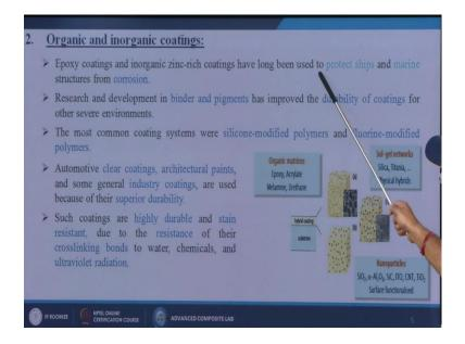
Next is that organic and inorganic coatings, so like epoxy coatings and inorganic zinc rich coatings have been used to protect ships and marine structures from the corrosion. Yes, if you remember i had talked about the antifouling, so what is that; when we are making any kind of submarines or maybe we are making any kind of ships, when it is
