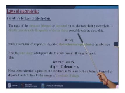
First one is called the Faraday's 1st Law of Electrolysis. So, based on these laws just we are doing the electroplating onto our sample. So, here the mass of the substrate liberated or deposited on an electrode during electrolysis is directly proportional to the quantity of electric charge passed through the electrolyte.
