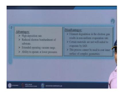
What is the advantages of this techniques? High deposition rate reduced electron bombardment of the substrate, because we are not going to disturb our substrate by any kind of electron bombardment so that it can change its shape and size; extended operating vacuum range, ability to operate at lower pressure. So, these all are the advantages for these particular techniques.
