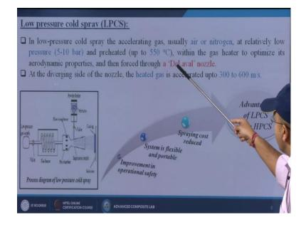
Then after mixing these two again it is coming through the DeLaval nozzle and directly it is depositing on to the substrate. At the diverging side of the module the heated gas is accelerated up to 300 to 600 meter per second that time it reached up to 1200 meter per second.
