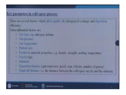
So, there are several factors which affect quality of cold sprayed coatings and deposition efficiency, what are those? First is called the gas type, what type of gas actually we are using, like helium, nitrogen. So, it depends that what is the substrate actually. So, the reactive gas it should not react with the substrate that we have to keep in mind. Then
