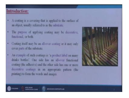
So, coating is a covering that is applied to the surface of an object usually referred to as substrate. So, substrate is nothing but the materials or maybe the metals which we are going to coat; so that is the best one. So, the thing is that either you can incorporate some materials inside the substrate so that we can do make a composites or maybe some kind of blends or maybe the alloys, but here without changing its chemical structure from
