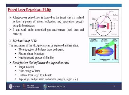
Next one is called the pulsed laser depositions or maybe the PLD process. So, a highpower pulsed laser is focused on the target which is ablated to form a plume of atoms, molecules and particulates directly towards the substrate; it can work under control gas environment both inert and the reactive gas. It depends upon which kind of material we are going to coat.
