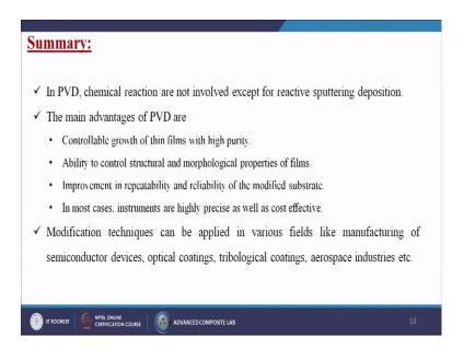
So, in PVD chemical reactions are not involved except for reactive sputtering deposition. So, here directly we are making any kind of gas or maybe the vapor then that is depositing onto the substrate.
