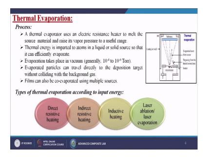
Thermal energy is imparted to atoms in a liquid or solid source, so that it can efficiently evaporate. Evaporation takes place in vacuum generally we are using the high vacuum because otherwise what will happen if we do not use the vacuum or maybe we do not use certain kind of inert gases maybe that vaporized materials can be reacted with the environmental oxygen or may be the moisture and it can form the newer materials or maybe the some un-useful materials.
