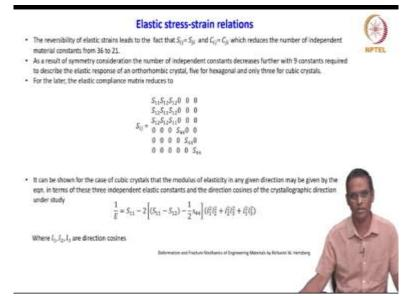
So, the reversibility of elastic strain leads to the fact that  $S_{ij} = S_{ji}$  and similarly,  $C_{ij} = C_{ji}$  which reduces the number of independent material constants from 36 to 21. So, we have also looked at the similar reversibility in the shear stress condition. Similarly, in elastic stiffness and compliance coefficient also the reversibility rule is applied and which further reduces the independent constants from 36 to 21 this is the point you have to remember.
