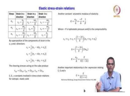
So, this is a table 3\* 3 matrix you can create using similar what we have just written there for a stress in x direction  $\sigma_x$ , we can write a strain in x directions
