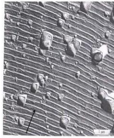
Fatigue striations on the etched failure surface in 2024-T3 aluminum alloy.
