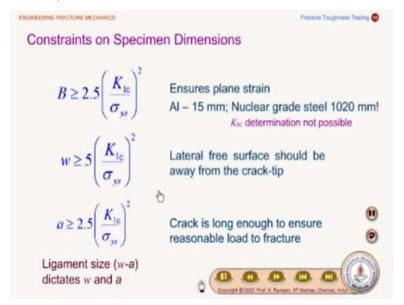
So now let us look at what are the constraints on the specimen dimensions, this expression we have already seen that minimum thickness of the sample should be B which should be equal to or greater than  $2.5(K_{1c}/\sigma_{ys})^2$ , ensures the plane strain condition. For aluminum alloy 15 mm nuclear grade steel it is a 1020 mm. So, this is very interesting to note you know so finding out the K  $_{1c}$  for such kind of thickness is not possible because of the conditions.
