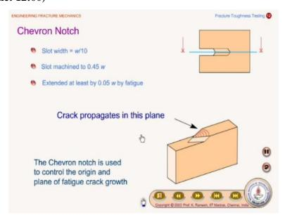
And this is just for a reference now I was just mentioning about this notch now we will look at what is the importance of this Chevron Notch the side view is like this and then slot with this w/10. And slot machine to 0.45 w and extended at least by 0.5 w by fatigue. So, this is why so to understand this geometry, let us, you should cut this specimen in the plane this perpendicular to
