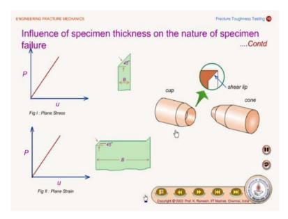
and the influence of specimen thickness on the nature of specimen again nature of specimen failure on this shear lip formation. So, this is for the plane stress condition and then this is a plane strain condition, you can see that this is a long and then finally shear lift formation takes place at this kind of setup.
