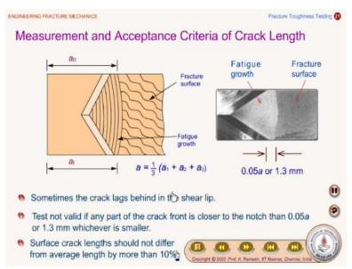
So now what we will do is? we will look at very important aspect, measurement and acceptance of criteria for a crack length. S,o, the pre-crack we have generated and then how to make sure that is really valid. So what you are seeing in this sketch is this is a crack growth region and this is done by fatigue free cracking and then this is a fractured surface this is you can see that actual specimen where you can see the fatigue crack growth region appears bright as compared to the
