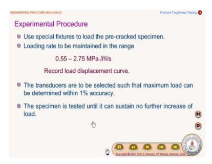
and saw the experimental procedures use special fixtures to load and the pre-cracked specimen loading rate should be maintained in the range of 0.55 to 2.75 mega pascal square root meter per second. Record load displacement curve that transducers are to be selected such that maximum load can be determined within 1% accuracy, the specimen is tested until it can sustain no increase of load it is like some simple pulling but with all the pre-conditions.
