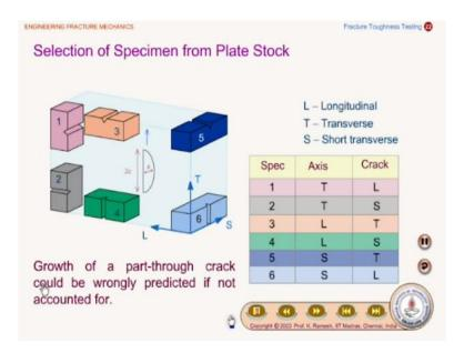
So, this is some recommendations about how to prepare this samples or how to take this samples from the material stock, to before we perform the test. So that is very important and this is also given in some of the codes but just to give an idea in a bulk material how to take the samples.
