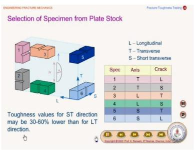
And how do we select the specimen from the stock there are some recommendations where there is suppose if you have the material stock of this nature then how do we take the samples and this is a table specification where we have an axis and they crack orientations are given that L is longitudinal, T is transverse and S stand for short transverse. So, toughness values for ST directions may be 30 to 60% lower than the LT direction.
