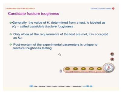
So candidate fracture toughness what is candidate fracture toughness generally the value of  $K_1$  determined from the stress is labeled as  $K_q$  called candidate factor toughness. So this is a test outcome and it will be recorded or declared as  $K_{1c}$  only after certain conditions only when all the requirements of the tests are met it is accepted as  $K_{1c}$ . So this is important post bottom of the experimental parameters is unique to fracture toughness testing.
