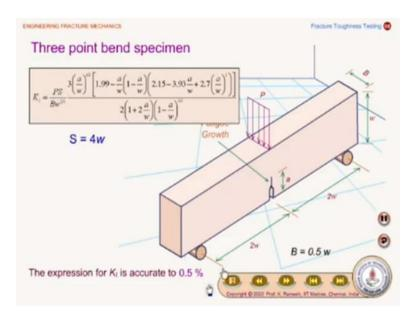
Next one is the three point bent specimen and we will have separate empirical relation for  $K_1$  as a function of a/W. And what is shown here is you know the dimensions are all shown here then we can just understand this expression for  $K_1$  is accurate to 0.5% in the range.
