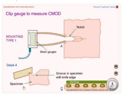
And what is to do noted now is how the clip gauges are fixed to measure the CMOD crack mouth opening displacement this is called a CMOD and typical gauge length, I mean the gauge is fixed here and this is a mounting type and this is chevron notch and this is a close up view how this gauges are fixed. And what we are trying to so now we will how the data is collected and.
