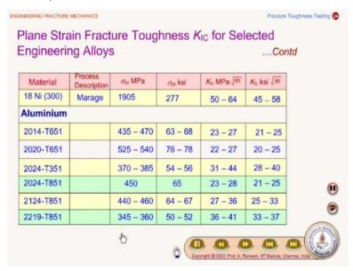
This is for non-ferrous alloys aluminum and you can see that strength levels are very different from the steel and then the K  $_{1}$  c value is also accordingly very different as compared to steel structures. Just give you a perspective about what kind of values one would expect in an engineering alloys.
