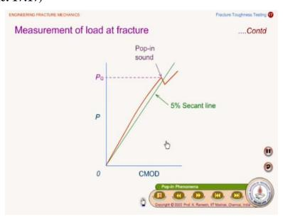
Then also there is a pop in sound phenomenon so in this case also you have the take the 5% secant line to take the P Q value this kind of load displacement data are normally obtained in the medium thickness specimens.
