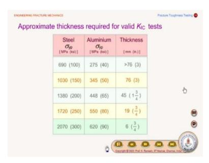
And we will just see the approximate thickness required for a valid K  $_{1\,c}$  test this is for generally steel it is 690 it is given in MPa and K  $_{1\,c}$  depending upon this and if it is of this range then the thickness is should be 76 mm or greater. Depending upon the  $\sigma_{yp}$  that is the yield point this values then this is also very that is that is constrained at least. For test common material like steel and material system here.
