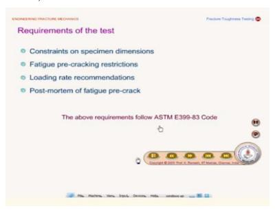
And the requirements of the tests are the following constraints on specimen dimensions fatigue pre-cracking restrictions and loading rate recommendations post-mortem of fatigue pre-crack. All these above requirements are even this ASTM code so it is quite elaborate details are given for this kind of important testing.
