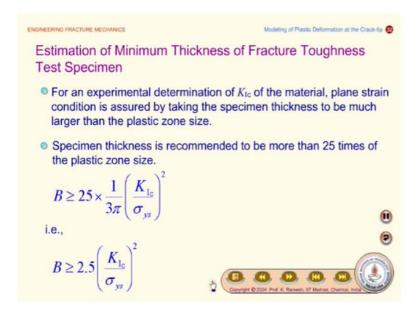
So how do we know? estimation of minimum thickness of the fracture toughness displacements. So if you want to this is going to be huge challenge now what is the minimum thickness for estimating the fracture toughness the displacement. For an experimental determination of  $k_{1c}$  the material plane strain condition is assured by taking the specimen thickness to be much larger then the plastic zone size this is first point.
