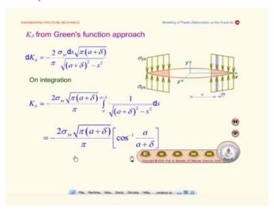
So  $K_{\delta}$  from Green's function approach so we will see what is that so the Green's function what is given here is basically the increment crack plastic zone and crack growth in the plastic zone is considered as a ds and this portion is taken as s. And then d  $K_{\delta}$ , is a given by this expression and then this is done I mean this expression is for the incremental growth ds. So if you integrate to the entire length then you will get the  $K_{\delta}$ .
