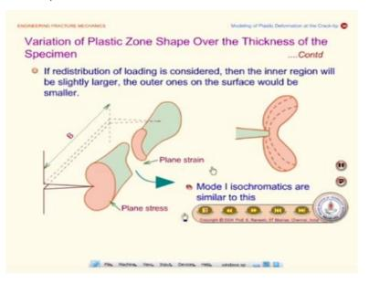
And if the redistribution is calculated and then again this plotted like this schematically though it does not give much difference between the re-distribution but nevertheless it gives the idea, I mean original idea into the same where the plastic zone size will be bigger on the surface that is
