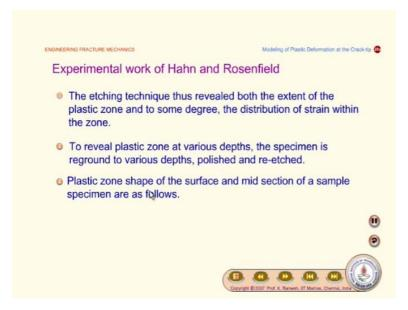
So, the etching technique does reveal both extent of plastic zone and to some degree of distribution of strain within the zone. So, the redistribution of the load is also being witnessed by
