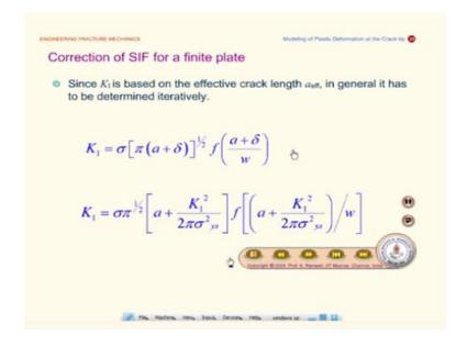
Corrective in the stress incentive called a finite plate so we know that now so far we have looked at finite plate and we will now come to finite plate. Since K  $_1$  is based on effective track length a effective in general it has to be determined iteratively. And K  $_1 = \sigma \left[\pi(a+\delta)\right]^{1/2} f(a+\delta/w)$ . So, this we have already seen you are not new to this it is a function of a instead of a by w it is  $a+\delta$
