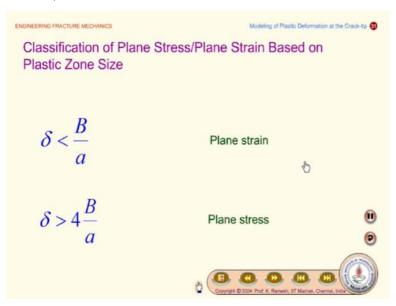
So now what we will do is, we will try to classify them classification of the plain stress and plain strain based on the plastic zone side. How, do we classify based on the classic zone size if  $\delta$  is less than B/a then that is belong to plain strain condition if the  $\delta$  is greater than 4 B/a, is the plane stress conditions. So this is one important idea to keep in mind.
