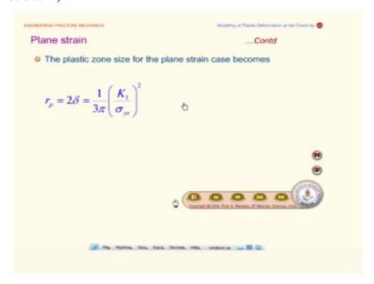
So the plastic zone size for a plane strain cases becomes finally  $r_p = \frac{1}{3\pi} \left(\frac{K_1}{\sigma_{ys}}\right)^2 = 2\delta$ .
