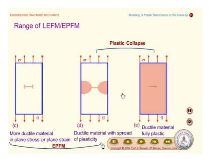
But the moment you go to very large plastic zone size for more ductile material in a plane stress or plane strain or you have the ductile material with spread of plasticity only with EPFM can handle this and of course elastic, when plastic collapse where ductile material fully plastic then these are not applicable whatever the idea which is discussed in earlier is not applicable to this. But up to this, these theories are calculations are valid.
