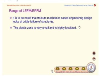
So if you look at what we already seen in the introduction slide, we have talked about range of LEFM and EPFM it is to be noted that fracture mechanics based engineering design looks at brittle failure of structure this is primary focus on fracture mechanics. The plastic zone is very small and is highly localized so this is assumption by which all the brittle material are handed by fracture mechanics that is the important point.
