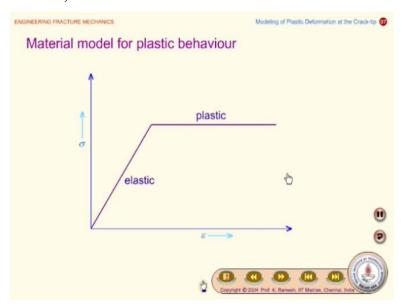
So, what is the material model we are considering a material model to be elastic perfectly plastic so that is how the materials is supposed to behave as per the, this model is concerned.
