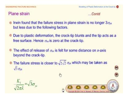
Irwin found that the failure stress in the plane stress is no longer 3  $\sigma_{ys}$  but less due to the following factors. Basically, it is correcting this simplistic model due to plastic deformation the crack tip bends and the tip acts as the free surface hence  $\sigma_{xx}$  is 0 at the character. So this is this point we have already seen when the crack tip is you know blunt by plastic zone then  $\sigma_{xx}$  is 0.
