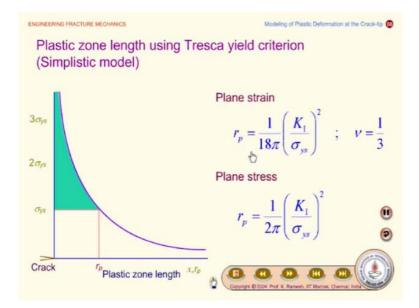
And then if you what will you get for a the plane stress condition  $\sigma_3$  is 0 so the  $\sigma$  is  $\sigma_{ys}$  so this is given by this  $r_p$ . So the plane stress condition the plastic zone  $r_p = \frac{1}{2\pi} \left(\frac{K_1}{\sigma_{ys}}\right)^2$ . So, you
