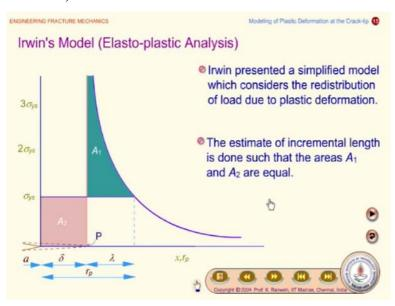
I will just, I want to replay this because I want to stop this first and then so I will just stop here then this is the, you know the load which is above the yield point which is not being considered in the previous analysis. So, this is the load which we are trying to redistribute and then try to recalculate the plastic zone length, so what happens? So that is how it is done so what is the methodology are been followed this kind of analysis which is shown in this.
