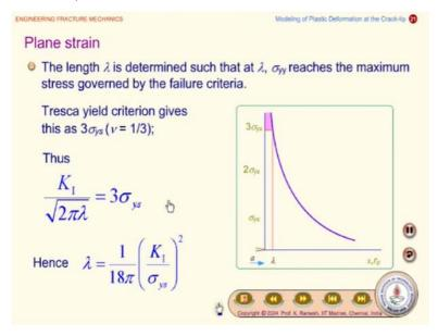
I mean, the first model given by Irwin the length  $\lambda$  is determined such that at  $\lambda$   $\sigma_{yy}$ , which is the maximum stress governed by the failure criteria. The Tresca yield criteria, give this has 2  $\sigma_{ys}$  like this we have seen earlier. So we can work it out like this  $k_1/\sqrt{2}$   $\pi$   $\lambda=3$  and this is already known. We have seen this already.
