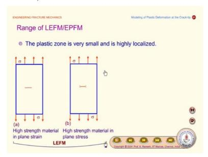
But when we say the plastic zone is very small what kind of plastic zone we are looking at, so this is some schematic which talks about where the high strength material in a plane strain condition and then high strength material in a plane stress condition so you can see that the plastic zone which is shown here is very very localized. But one very important to note is the plastic zone in the plane strain is much smaller as compared to a plane stress situation.
