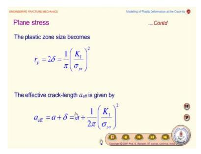
So the plastic zone size becomes  $r_p = 2 \ \delta$  which is equal to  $1/\pi (k_1/\sigma_{ys})^2$ . So the effective crack length a effective is given by  $a + \delta$  which is nothing but  $(a + 1/2\pi)(k_1/\sigma_{ys})^2$ . So this is very you know a very useful information because this Irwin's considers the redistribution of the load. So the effective crack length you know which is very important in calculating the stress intensity fact has been arrived by first approximation.
