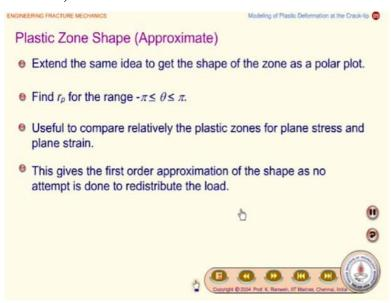
So how do we understand the shape it is very quite difficult that is why it is written as approximate. Extend the same idea to get the shape of the zone as the polar plot so we that we can represent  $r_p$  in the range of  $\pi$ , I mean  $\theta$  can be expressed in between  $-\pi$  to  $+\pi$  and useful
