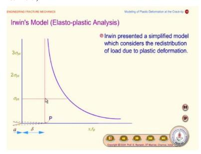
The first one is Irwin model which is also considered as elastoplastic analysis. Irwin presented a simplified model which considers the redistribution of load due to plastic deformation. So how the redistribution of model is done just look at this plot, the same plot  $\sigma$  versus r  $_{p}$ . And if you look at this where the yield stress is considered.
