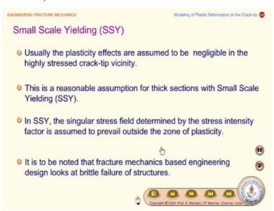
So in this context we also mentioned in the production something called small scale yielding what is small scale yielding? Usually, the plasticity effects are assumed to be negligible in the highly stresses crack tip vicinity and this is a reasonable assumption for a thick sections with small scale yielding is called SSY. In SSY the singular stress field determined by this stress intensity factor is assumed to prevail outside the zone of plasticity.
