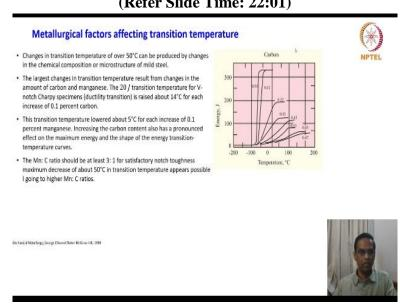
Just finally what are the important metallurgical factors affecting the transition temperature very important. Changes in transition temperature of over 50° can be produced by changes in the chemical composition or microstructure of mild steel, this is just one example. So, what is the message by tweaking the chemical composition or by doing a proper alloy design or microstructure that is proper pre-treatment, you can have a control of transition temperature
