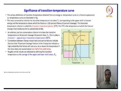
So, what is the significance of this transition temperature curve, the various definitions of transition temperatures obtained from energy versus temperature curve or the fracture appearance versus temperature curve are illustrated in the figure. You see, since I said the test is quite simple people have known adopted different terminology to identify the fracture behaviour of materials.
