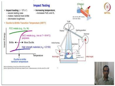
Hello, I am Professor S. Sankaran in the Department of Metallurgical and Materials Engineering. Now, we will move on to another basic mechanical testing called impact testing, very important industrial setup and very old testing methodology especially after the grand failure of liberty ships and another catastrophic failures which, I mentioned in the beginning of the course, this test becomes quite popular to assess the ability of the material to undergo brittle fracture and so on.
