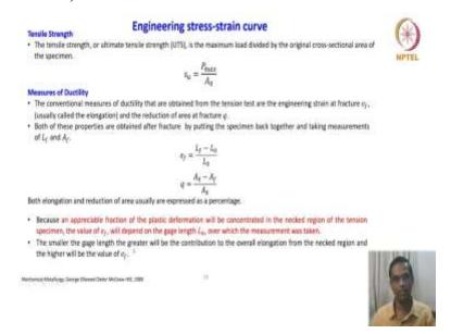
Hello I am Professor S. Sankaran in the Department of Metallurgical and Materials Engineering. So, we will now go to another parameter called tensile strength that is the tensile strength or ultimate tensile strength UTS the maximum load divided by the original cross sectional of the specimen which is called also called tensile stress is a maximum load maximum strength which is given by  $S_u$ , S is engineering stress u is ultimate which is  $P_{max}/A_0$ .
