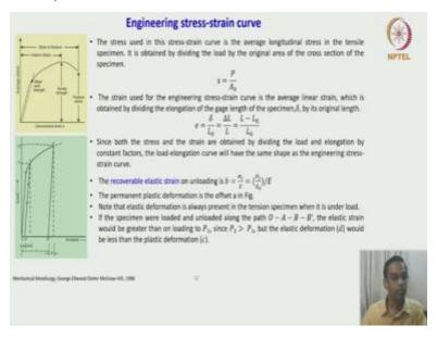
So, normally in any textbook, the engineering stress strain is illustrated like this. So, what is plotted here is an average stress versus conventional strain. So, you can see that the average stress goes like this and reaches a maximum and it comes down, the stress used in this sustained curve is the average longitudinal stress in the tensile specimen. This is obtained by the load by the original area of cross section of displacement.
