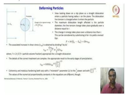
So, this is a schematic which shows that the deformable nature, so the dislocation line is there and it is moving in the matrix and this is a precipitate and the precipitate experiencing the dislocation entry and this is the line tension of the dislocation is altered and it is maximum when it goes to the distance radius here for the change in the line segment energy is driven by  $\frac{(\mathbf{G}\,\mathbf{p}-\mathbf{G}\,\mathbf{m})\mathbf{b}2}{2}$  (2r)
