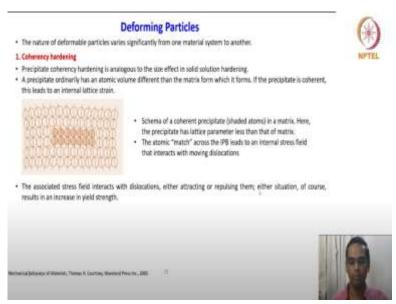
First, we will discuss about deforming particles. We are going to talk about particle hardening and in the first cases deforming particles. The nature of deformable particles varies significantly from one material system to another, which one is characteristic. In deforming particles, we will first discuss about coherency hardening. What is coherency hardening? Precipitate coherency hardening is analogous to the size effect in solid solution hardening.
