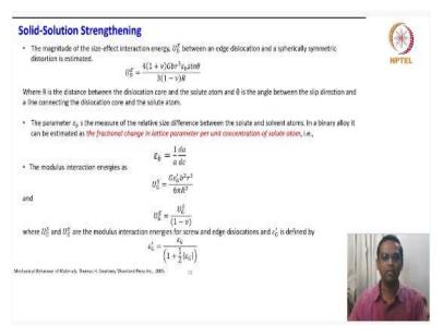
If you look at the magnitude of size effect interaction energy that is  $U_D^E$  between the edge dislocation and a spherically symmetric distortion is estimated. Which is given by this expression
