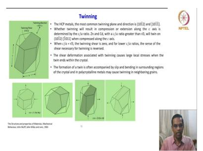
So, this is one illustration of HCP unit cell where you see that the lattice parameters are not a and c and this is a  $(10\overline{1}2)$  twin plane and this is  $[10\overline{1}\overline{1}]$  of family of twinning direction. So, these are the most common twinning plane and direction in HCP metals. And but you have different situation here in HCP metal it is very interesting whether twinning will result in compression or extension along the c axis is determined by the c/a ratio.
