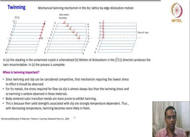
We will look at one more illustration regarding this mechanical twinning mechanism in an BCC lattice by an edge dislocation motion, this hypothesis can be understood by another illustration here, what is that you are seeing it is these are all a stacking and untwined crystal is shown in this schematic and this is  $[\bar{1}11]$  direction and then this is the a trace of 112 in a BCC in BCC, you have this trace 112 for twinning.
