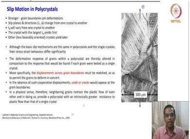
Slip motion in polycrystals so, now we looked at the basic mechanisms of plastic deformation called the slip and twinning in single crystals and then we looked at all the all possible I mean
