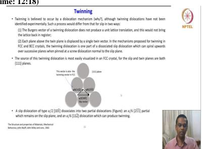
So, twinning is believed to occur by a dislocation mechanism although twinning dislocations have not been identified experimentally, we have to ask the question here. Why do we believe that it has to occur by a dislocation mechanism if you recall when we just looked at a perfect single crystal, we also looked at the theoretical you know strength of a perfect crystal. And if you assume that twinning also takes place without a dislocation or without any assistance of the dislocation.
