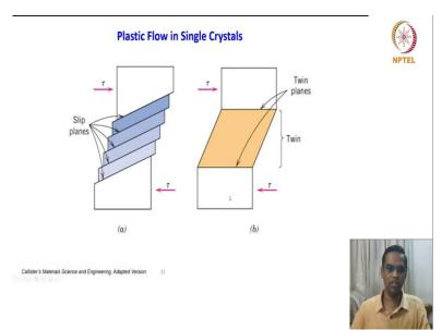
So, if you look at the plastic flow in a single crystal, so this is how the crystal will slip and then we can look at the slip planes the slip plane will appear like this against the shear force direction and each one will have the you know the slip planes may not be uniform like this it could be randomly I would say that it is a random aggregates of the slip plane will appear with the non uniform distance between them.
