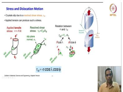
And then we will see how dislocation proceeds, dislocations proceeds so, because of the two aspects, first is because you are applying a load, which is measured as stress and because of that the dislocation moves in the crystal that is the primary action that takes place result in the deformation. So, this is a schematic which shows where we applied we apply the tensile force is F and the cylindrical member is getting slipped.
