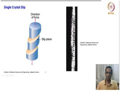
And this is a single crystal metallic's which you can see that the real time experiment which is given in this text I just brought to give an example how the slip planes exactly looking like what we have just shown in this schematic the real time slipped regions will exactly look like.
