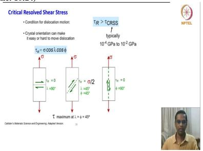
So, this is it is not that the resolved shear stress of any quantity will cause slip there is something called critical resolved shear stress that means, it is a kind of condition for dislocation motion, if you recall we have also seen that a stress required to move or dislocation suppose number equation if you recall it something similar to that you can you can relate that.
