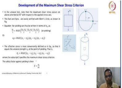
So, how to develop this criterion in the uniaxial tests note that the maximum shear stress occurs on the planes oriented at 45 degree with respect to applied stress. This fact and equation are easily verified with Mohr's circle as shown in figure, so this is just to reinforce our understanding not that anything we are finding it new here. Just plot this ideas into a Mohr's circle and we will get to know see the visual experience of the maximum shear stress criterion.
