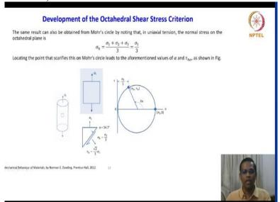
So, again we will plug in all this values into the Mohr's circle the same result can also be obtained from Mohr's circle by noting that in uniaxial tension the normal stress on the octahedral planes is nothing but  $\sigma_1/3$ . Locating the point that sacrifices are Mohr's circle leads to the aforementioned the values of  $\alpha$  and  $\tau_{h0}$  how do we do that. So, this is again
