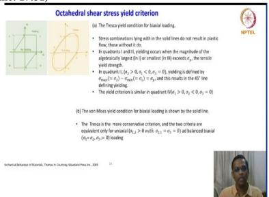
Now come to be the most important idea we are now created the surfaces the yield surfaces or the fracture surfaces here it is yield surfaces for biaxial loading, this is a shear stress yield criterion and which shows that four quadrants I II III IV and then you have  $\sigma_1$  and  $\sigma_2$  and the boundary demarks are no yielding and then yielding. Stress combinations lying within the
