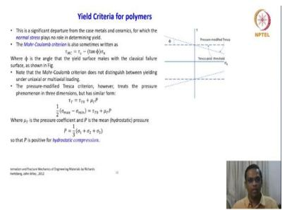
So, this is a significant departure from the case of metals and ceramics for which the normal stress plays no role in determining the yield so very important idea, where we are bringing a normal stress into any especially a stress yield criteria. So, what is that we have seen so far interest gap. So, this is what this part shows clearly this is a normal Tresca yield threshold is shown in a dotted line here a thick dotted line and this is  $\tau$  and this is  $\sigma_n$ .
