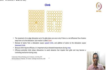
So, finally the we talk about climb we have already discussed this in terms of dislocation motion and here the schematic shows the extra half plane in one case it is extending downward the other case it is moving upward. So, there are two possibilities either it can
