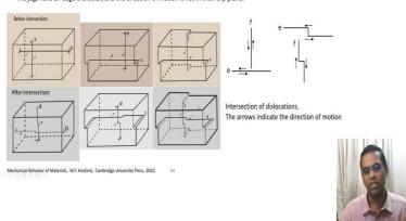
So, this is the figure we were referring in the previous slide. So, we will concentrate one by one there are too many figures at one time. So, it is better to spend some time to understand the figure first and then we will get into the concept the unit cell which is drawn here this is before intersection. There are two dislocation lines are drawn a and b if you look at the a the edge you can clearly see that edge dislocation side.
