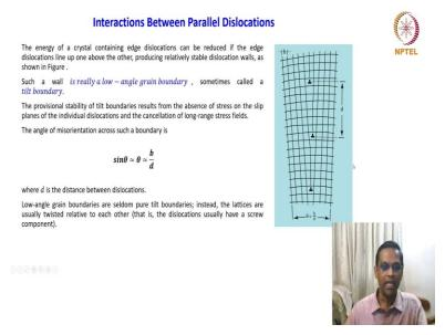
So, the energy of the crystal containing edge dislocations can be reduced, if they edge dislocations line up one above the other produces relatively stable edge dislocation walls as
