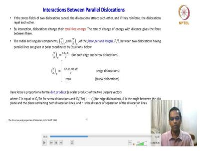
So, we are going to continue that idea today, so interactions between two parallel dislocations. So, we will just look at the concepts which we have already seen in the last class. It will be a slightly redundant here but it is still looking it is kind of a revision in the stress field of two dislocations cancels, the dislocations attract each other and if they reinforce the dislocation repel each other. So, by interaction, a dislocation changes their total free energy.
