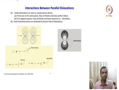
So, what is the next one unlike dislocations on the same a nearby plane attract? So, this is quite obvious this schematic should be wrong because the unlike means the T should be up and C should be down. So, there is a correction here and because they should compare this symbolism here this is positive dislocation, this is negative dislocation so it should be rotated 90 degree. So, there is a correction here.
