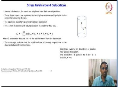
So, around a dislocation, the atoms are displaced from their normal positions, these displacements are equivalent to the displacements caused by elastic strains arising from the external stresses. So, to describe these stress fields and then this is a coordinate we are choosing just a reference and you can see that polar coordinates. So, these coordinate systems for describing your location near a screw dislocation.
