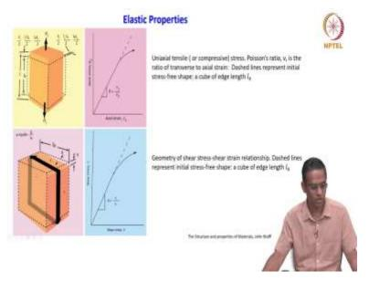
So, the diagrams which are going to show now is going to explain geometrically whatever we have just seen in terms of you know the elastic this is a member which undergoes tensile deformation. So, you see that  $l_0$  becomes 1 after the deformation and then you see that change in length and then you try to calculate the displacement and then from there to calculate the stress and strain.
