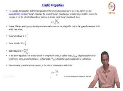
Hello I am Professor S. Sankaran in the department of metallurgical and materials engineering. For example the equation for the linear portion of this tensile stress strain curve is
