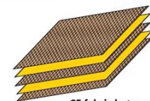
CF fabric between metal sheets for diffusion bonding
