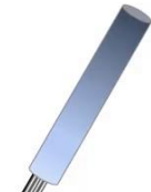
Carbon fiber bundle in a glass capillary for biosensing
