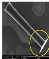
Non-uniform shrinkage in structures attached to substrate
