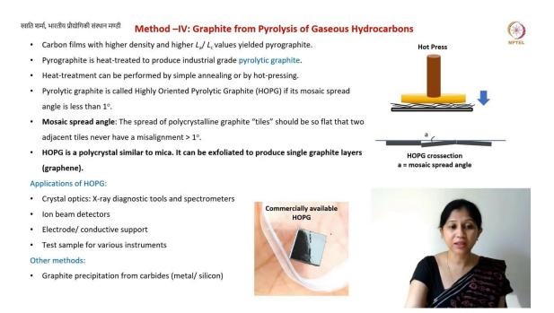
Now we come to the method of making graphite from this pyrolytic carbon or pyrographite. If it has a very poor density and poor crystallinity, we will just call it pyrolytic carbon but if it has a reasonable La and Lc value, then you will call it pyrographite.
