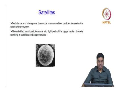
Then, we also discussed about a problem in this process which is known as satellites that occurs due to turbulence and mixing near the nozzle and satellites are smaller particles which stick onto the surface of bigger particles and make the surface rough. So, this is a small problem which might occur during the process of gas atomization.
