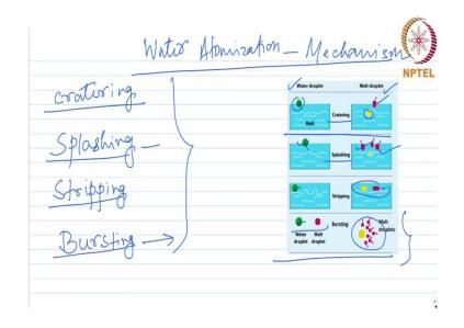
Here also there is a particular mechanism through which the fine droplets are formed from the molten stream of the metal. The mechanism has been depicted in this particular diagram; primarily there are four ways or four kinds of mechanisms through which these droplets of the metal forms with the help of a water jet.
