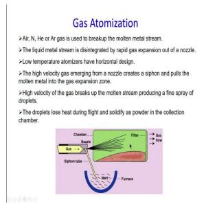
And then we have discussed about two different types of equipment which are used for gas atomization, for making metal powders; one of these is a horizontal design where you can see here the chamber is horizontal.
