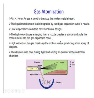
So, the first one we are going to take up is Gas Atomization; wherein you use this gas jet as a mechanical force to disintegrate this molten metal stream into finite droplets. So, this we have seen before also, how actually this gas, this high velocity gas jet, how it actually helps in breaking down this molten stream of metal into fine droplets.
