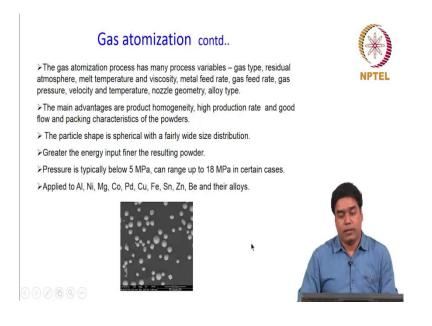
So, now for this gas atomization process if you see the process variables; there are many variables in this process like the gas type, for example, different types of gas like air, nitrogen, helium or argon can be used and they will have their own effect on the process. So, the type of gas which is used is a process variable.
