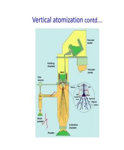
So, in that case the chamber is vertical and the flow is vertically down.
