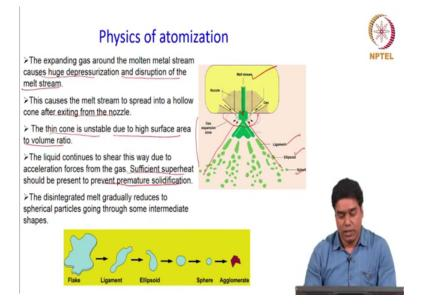
So, this is how the process is in terms of the phenomena or the principle. If you see it, we will take an example here of the gas jet, which is used to atomize the molten stream of a liquid metal ok. So, what do you have here? You have this chamber in which you have the molten stream coming through. And this molten stream of metal is sent through an opening like this through a nozzle and where, the nozzle exit is at that location you have this high velocity gas jet coming in .
