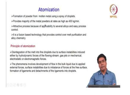
So, as I said you know the formation of powders from molten metals using a spray or droplets . And this is a process which actually provides the majority of metal powders
