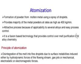
The phenomena involves development of flow in the bulk liquid due to applied external forces, surface instabilities due to imbalance of forces at the free surface, formation of ligaments and detachments of the ligaments into droplets.
