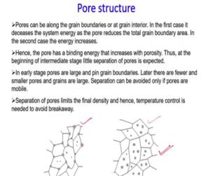
So, when the pores will finally, you know distributed in the material they can be either along the grain boundaries or at the grain interiors. So this is one picture which shows that the pores are the primarily along the grain boundaries right and here the second one shows the pores to be primarily located in the grain interiors.
