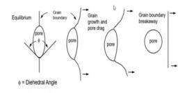
So, talking about this interaction between the grain boundaries and the pores, we can depict it with a diagram like this. So, for a pore sitting on a grain boundary the equilibrium between the grain boundary energy and the solid vapor surface energy will cause a group to form as you could see from here and the angle of this group is known as the Dihedral angle . So, that is how the interaction between the pores and the grain boundaries will start.
