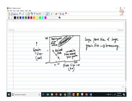
It can also be shown by a plot between grain size and pore size. So, if the grain size is plotted against the pore size then it will look something like this, it will basically help us identify the region in which the breakaway of the pores will take place.
