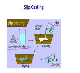
This is a schematic of the process as to how the slip casting process is carried out; a slurry or a suspension is first met, and then that suspension which is also known as a slip is poured into this kind of molds which are porous in nature. So, these pores absorb the liquid and the powder particles will take up the shape of the mold cavity.
