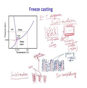
The process of removing the water has to be carried out below the triple point. The water phase diagram which is also known as the pressure temperature or P-T diagram (above graph in the image). Wherein, you can see the 3 states of water. The diagram depicts which particular state is stable under which conditions of temperature and pressure.
