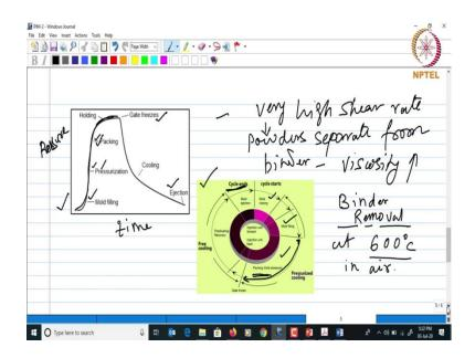
Now successful molding also requires low viscosity and viscosity will depend on the shear rate. If the shear rate is very high then the powders will tend to separate from the binder and the viscosity will increase and it will lead to non uniform mold filling because the mold filling depends on availability of a fluid mixture which can easily flow into the cavity to all the corners.
