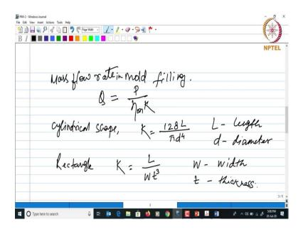
Now, if you look at the mass flow rate during the mold filling, that is also an important parameter that has to be looked at. Let us call that as Q and the relation of Q with the pressure P is given as this:
