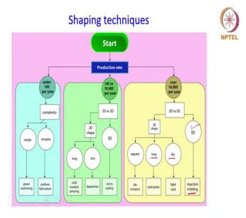
Now, let us come back to this diagram where it all started. So, from here you can see what kind of shaping techniques are needed for what kind of shapes and you can see injection molding is over here and it can be used for making 3 D shapes and complex shapes.
