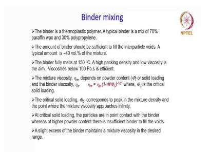
So, let us first talk about the binder mixing process before we actually go to the molding process because this is the first step. The binder basically is a thermoplastic polymer. A typical binder is a mix of seventy percent paraffin wax and thirty percent polypropylene. And the amount of binder should be sufficient to fill the inter-particle voids. A typical amount is about 40 volume percent of the mixture.
