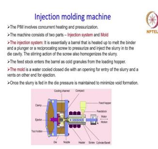
Now, let us see how this injection molding cycle goes. Powder injection molding involves concurrent heating and pressurization. If you look at the machine it basically consists of two parts, the injection system and the mold. The injection system essentially is a barrel that is heated up to melt the binder and apart from that it has a plunger or a reciprocating screw which is used to pressurize and inject the slurry into the die cavity, ok. So, the die cavity is the other part which is the mold.
