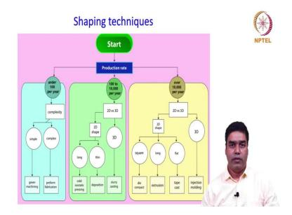
Now, there can be more complex shape parts where it is all the more necessary to maintain the uniformity, during the compaction process. So, as you can see from this diagram (slide above) powder injection molding is a process which can handle complex shapes including 3D parts and this is what we are going to discuss next.
