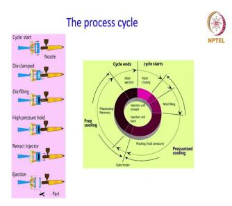
So, this is a schematic (slide above) which shows the process cycle from the start of the process to the end. At the start of the cycle the nozzle and the mold cavity (that is the injection system), and the die cavity, these two are kept ready and then the die is clamped and it is steady for the die filling process.
