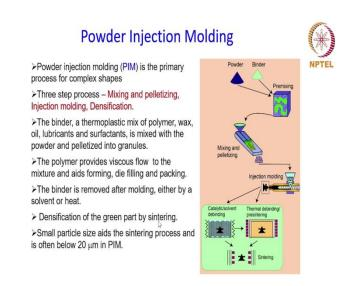
Powder injection molding is a process which can make complex parts including 3D parts, as we have seen before in that diagram which talks about the different categories of the shaping processes depending on the type and shape of the part. Powder injection
