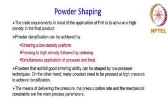
Several methods are available to shape and form powder. A particular method is selected based on the requirements in the final product.
