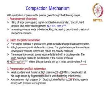
Now, going into little more detail into the compaction mechanism, let us see what happens during each of this phenomena that we described in the previous slide. With the application of pressure, the powder goes through the following stages and the following phenomena as we have seen in the previous slide also.
