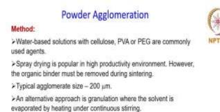
So, far this spraying or the atomization process, water-based solutions with cellulose, polyvinyl alcohol or polyethylene glycol are commonly used agents. Spray drying is
