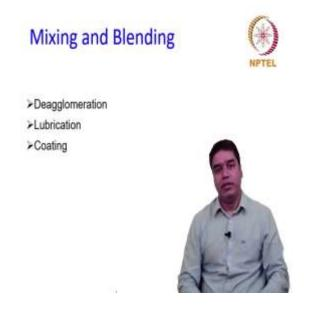
So, with regard to the preparation of the powder feedstock for the shaping process, there are few more things that we need to discuss and these are as follows. Deagglomeration of the powder, powder lubrication and powder coating. So, let us go ahead and discuss about these aspects of the powder feedstock preparation.
