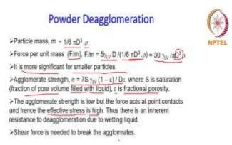
Now, if you consider the force per unit mass, let us say we are talking about a spherical particle. The mass of a spherical particle will be given by
