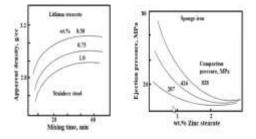
Now, let us see what are the benefits of powder lubrication. First of all the apparent density will increase and you can also see that in terms of the mixing time, which is shown over here in this diagram. The apparent density increases with the mixing time, the mixing time that is allowed for mixing the lubricant with the powder.
