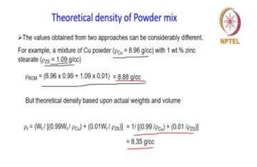
One thing that you should note over here is that, the values obtained from these two approaches can be considerably different. For example, if you consider a mixture of a copper powder and 1 weight percent zinc stearate, which is used as a lubricant. The respective densities are given here for copper and for zinc stearate and now if you calculate the theoretical density based upon the rule of mixture, this will be simply given by this.
