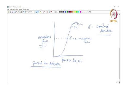
And it is typically an 'S' shaped curve like this and from this you can also derive the statistical information like the median size corresponding to  $\sigma = 0$ ,  $\sigma = 1$ ,  $\sigma = 2$  and so on where sigma is the standard deviation.
