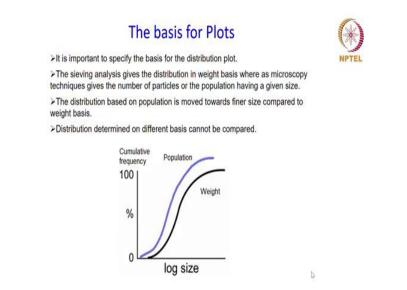
And one thing I must mention over here is that when you are representing the cumulative plots, it is important to specify the basis for the distribution. The data collection can be a population based or it can be weight based.
