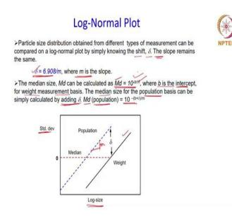
It will give you a straight line. And now, in order to compare the data which is collected from different using different basis, this is what you can do.
