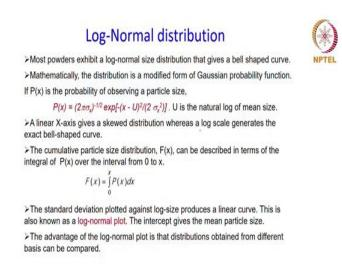
Cumulative plot is a summed up representation of the data. Here too, the data is summed up from a particular size to a given size, x, or over a particular interval from 0 to x.
