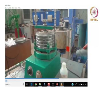
Once the shaking motion is given, the powders will go down through the screen depending on the size of the particles.
