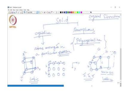
So, if you talk about a solid material in terms of its internal structure which is also referred to as the crystal structure, there are two kind of solid materials, two categories that the solid can be broadly categorized into depending on the crystal structure; one is a Crystalline and another is Amorphous.
