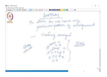
In this case the atoms do not have any particular pattern of arrangement or in other words, patterns are arranged randomly right. So, these atoms, they may not have to follow any particular order like what we have seen in case of the crystalline materials. So, there is no repeating of any of these features or distances in a periodic manner, when the structure is amorphous .
