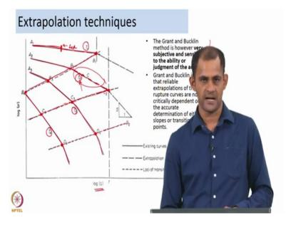
So I will just use this graph to explain what I am trying to say here, so this is a graph that is use by Grant for using the Grant-Bucklin method. So you have log sigma Versus log t r, so the time to rupture changes as a function of sigma for different temperatures, so you have T 1, T 2, T 3 and T 4, so if you see there is a change in slope depending on the applied stress temperature and time.
