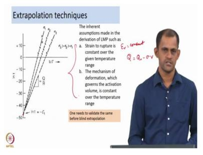
So that is what I am showing in this particular slide, is you can plot log t r Versus 1 over T for different values of sigma and they all intersect the Y axis at the same location and this gives you the value of c which is the constant in the Larson-Miller parameter equation. Now one
