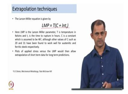
So the Larson-Miller parameter is given by the following equation, so LMP which is Larson-Miller parameter is dependent on the temperature and time to rupture and T is generally taken in kelvins and tr which is a time to rupture is taken in hours, C is a constant which is generally assumed to be 46, all the other values of C such as 20 and 31 have also been found such as for example 20 steel in austenitic steel and 31 steel in ferritic steels.
