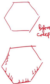
Dislocation activity close to a grain boundary in a Ti alloy crept in the grain boundary sliding regime
