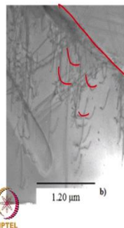
Dislocation activity close to a grain boundary in a Ti alloy crept in the grain boundary sliding regime
