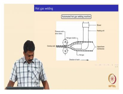
We will move on so we can also automate the process to make the longitude seen joints, again the principle is the same as we do in hot plate welding, the only thing is here we add a blower and then a filler, it can be sent to the joint subsequently can be filled the rollers can
