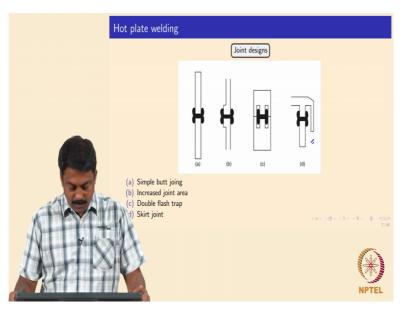
So what are joint design we commonly use for hot plates? Simple label joint and you can also increase the area okay so that the well strength and joint strength increases at that regime and you can also do double flash and skirt joint okay, so this skirt joint is also commonly used for polymers right, good so we will move on, so we will just run through.
