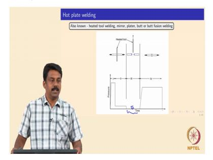
Okay it is also known as hot tool welding or mirror, platen, butt and fusion welding processes, so the method is very simple in hot plate welding so you have one heated tool or plate that goes actually inside the (())(6:05) interface to join right and then you melt the interfaces right so you have heated tool, the joints to be welded or heated up at the interface using an hot plate and subsequently apply in (())(6:25), so you also create some scene.
