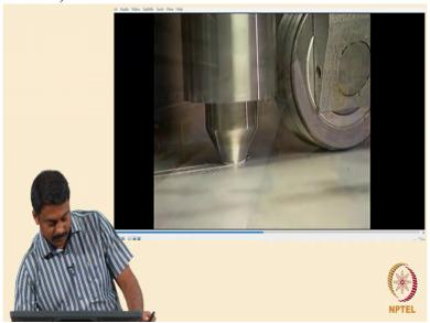
So we will see this process. So this is the shoulder, what you look at it. Ok shoulder is extending and then pin is plunged into the base material. And it is rotated causing mechanical
