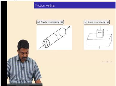
And we can also make it in a, in the heat generated, friction generated in various ways isn't it? For example we can also make it angle reciprocating friction welding. So instead of doing continuous rotation we can also do reciprocating motion, right.
