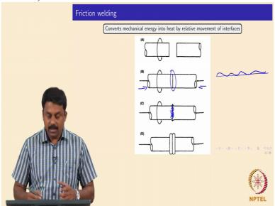
the inner interface is going to coalesce to form a joint, isn't it?
