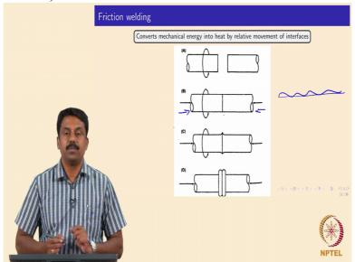
So this interface is going to heat up, isn't it? So once it heats up because of the upsetting force you are supplying you will have a mechanical deformation at the interface.
