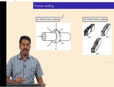
so in this case the force is applied perpendicular to the loading direction or rotation directions.
