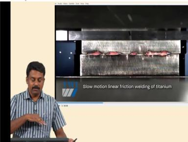
you steadily increase the force and then we also control the amplitude of reciprocating motion. So the interface heats up by the friction heat. So you have mechanical deformation.
