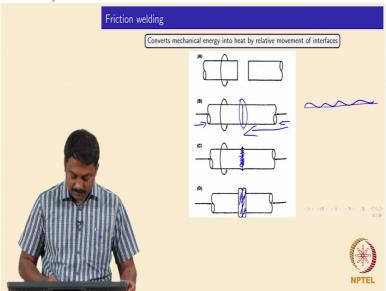
So once you machine it off, it will be a complete joint made. And the joint would have a much better mechanical properties than when you are doing in a fusion welding.
