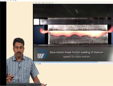
the orbital motion so that you can heat up much faster. And then upon increase in temperature you keep it for some time with the pressure so that the weld would be completed. Yes, it is clear?
