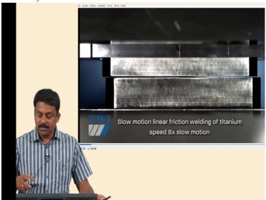
as we said, is very commonly used for welding superalloys and (()) (31:59) titanium blades to the blisk
