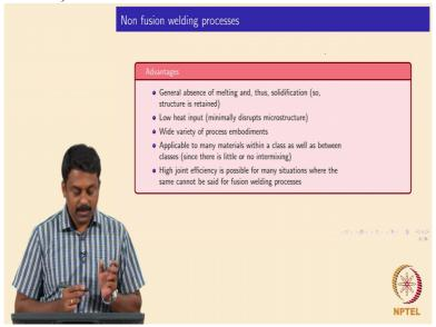
the concept of solidification is gone. You do not have solidified microstructure, Ok. So you will have a mechanical deformed and recrystallized microstructure isn't it?
