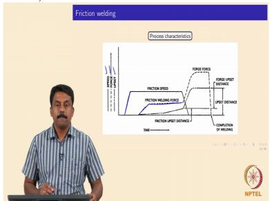
and then the moment the temperature is reached to required temperature, increase of force on the upset.
