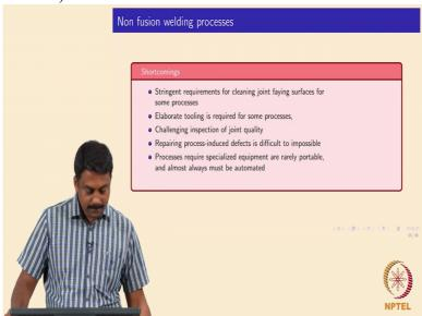
So what are the disadvantages of non fusion welding processes? The interface in most of the cases should be cleaned properly.
