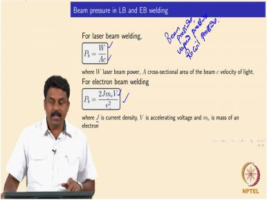
So the keyhole again formation is the same as laser beam welding. Right? So the (())(10:23) that 8 kilowatt formation beam pressure, vapour pressure and then recoil pressure. In electron beam welding process, the beam pressure is much wider than laser beam welding. So in a way, it is
