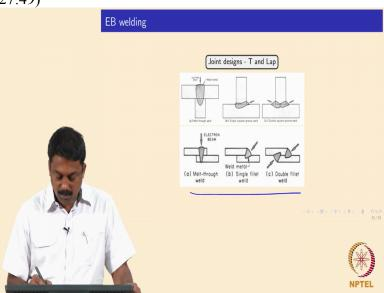
And some other configurations, so ya the T joint and L joint and it is very well done in electronbeam welding using a melt through configuration. Whereas in other joints, so you will have to do a single groove or double groove T joints. In electronbeam, you can achieve a simple melt through welds. So if you want to use GMAW, so you will have to use a single filled welds or double filled welds to achieve similar weld configuration. Yes. It is clear? Any questions?
