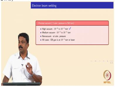
So in the most of the cases we need to maintain a very high vacuum. So nowadays we also have an atmosphere system. So but it is not really atmosphere system. The we still have electron gun but the Sample can be in atmosphere. So the in all cases, the electron gun should be at a very high vacuum. Okay. But you can make sure you can develop a system in such a way that the
