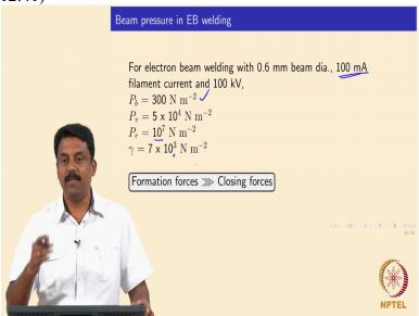
And if you look at the beam pressure of the electron beam welding, it will be much higher. Right? The beam pressure in electron beam welding it will be close to if you do a simple mathematics using target current of 100 milliamperes and then the isolation voltage of 100 kV and we can achieve the beam pressure of 300 newton per metre square. So that is 300 newton square. Okay. That is huge, the beam pressure itself. Okay. So it is acting.
