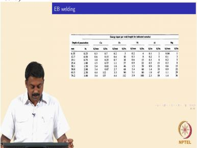
So this table shows the energy input we use and what depth of penetration we achieve for a given ya composition of material. So for example in copper, the energy we what we need is kilojoules per millimeter. Okay. So (())(28:46) reference table which you can use it.
