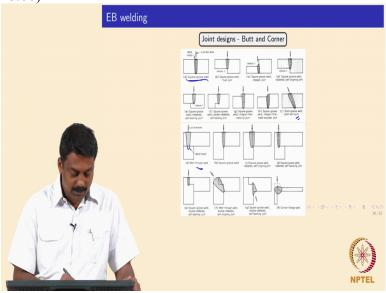
So the most preferred joint design is the square groove butt joint. Okay. And all the configuration if you look at it, it is the manipulation of the butt joint only. Okay. So we can have a slightly inclined butt joints but in most of the cases all these butt joints in varying configurations you can achieve. And we see over here, melt through weld and this is can be this can be achieved only by electronbeam. Okay. So it is like you know you join two and you are not doing filled weld.
