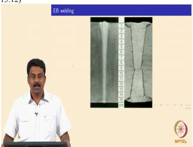
So the keyhole shape would always be like this. So what you see over here, so this is 15 centimetre, it is not millimetre. Okay. So that is 150 millimetre. And you see, we can achieve full penetration of 15 centimetre and you could have full penetration of 150 millimetre. So once the millimetre, 15 centimetre, something like this of steel. Okay. And you can have complete penetration in a single pause. Yes?
